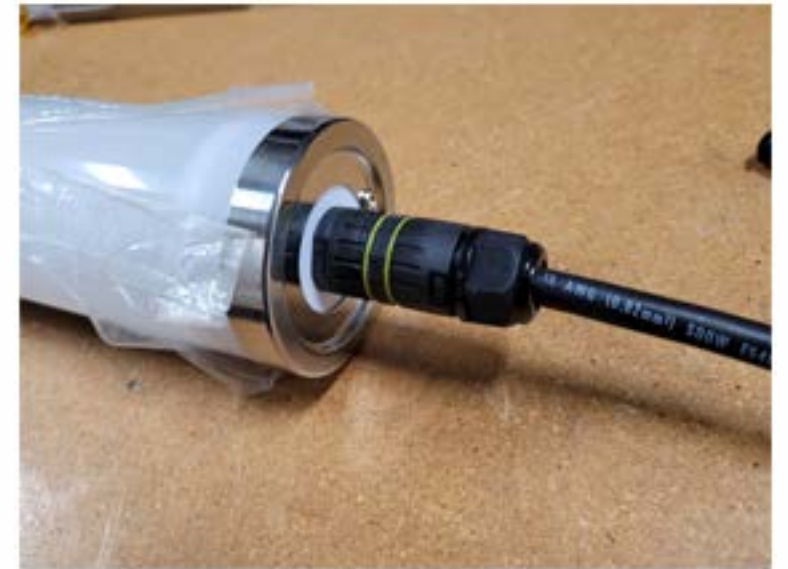
6. Completed power cord installation
