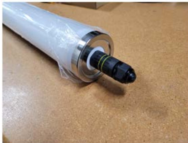
8. Completed installation of plug
