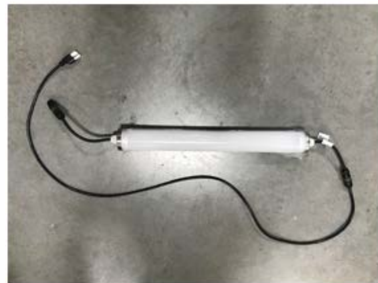
11. Connectors added to existing power cords.
